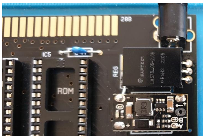
Switching voltage regulator and mini step-up module on an Issue 3b board
